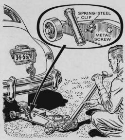
**Flashlight Helps Spot the Jack.** A flashlight clipped to the side of a shop jack like this will help locate the jack under a car, especially when light is bad. The clip can be screwed to the jack frame or tack-welded in place.
