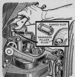
Removing Shock-Absorber Plugs. On some shock absorbers the head of the filler plug is recessed. If the corners of the hexagonal plug head round off, you've got a problem. A socket wrench won't hold. One solution is to hacksaw through one side of a spare socket, slip it on the plug, and squeeze it tight with a vise-grip wrench.
