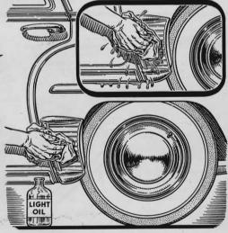
How to Protect Chrome. To prevent rust, apply light oil after each washing and wipe away surplus. The American Electroplaters Society recommends such washing and oiling at least three times a winter if salt is used on highways. To remove rust that has formed, use any scouring powder that is safe on porcelain or tile.
