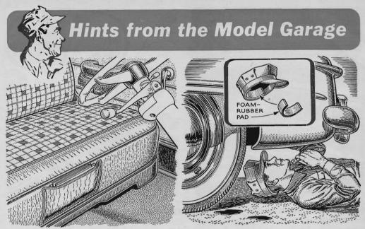
Unloading the Glove Compartment. A pocket sewn to the seat cover like this makes a handy place to keep maps and other bulky papers. Centered, it won't be in anybody's way. For appearance, try to make it of the same material as the covers.
