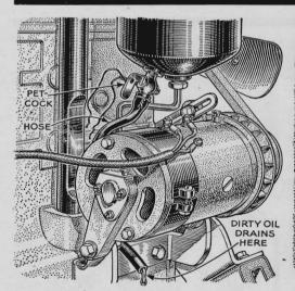
Hose Drains Oil Filter. Many oil filters have a plug at the base for draining out sludge and dirt. If the drainings would fall on engine accessories below, install a petcock like this and run a synthetic-rubber hose down far enough so the dirty oil will drop clear. Drill a hole in the petcock handle and use a wire to "safety" it.
