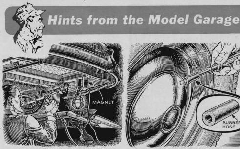
Magnet Supports Light. By looping an extension cord around a large horseshoe magnet, you can place a light exactly where you want it while working under a car. It's handy in places where the hook support doesn't spot the light where you need it.
