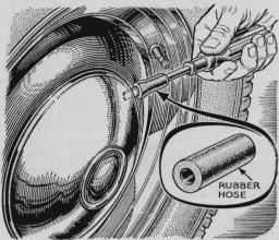
Rubber Prevents Paint Scratches, A short piece of rubber hose slipped over your screwdriver will protect wheel finish when you're removing hub caps. Slip the tip under the cap and slide down the hose as far as possible before you pry.
