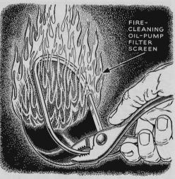
Fire Clears Stubborn Screens. Your oilpump screen should be cleaned occasionally, even if you must drop the pan specifically for the purpose. If brush and gasoline won't do the job, put a match to the screen, let the sludge burn, and brush away the ash. This won't damage a screen unless it's soldered together.
