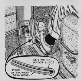
**Slit Hose Protects Trim.** On the interior of a car, one of the first points to show wear is the beaded trim at the doors. To repair such wear, or prevent it, slit a short piece of hose and slip it over the trim. The elasticity of the rubber will keep it in position.
