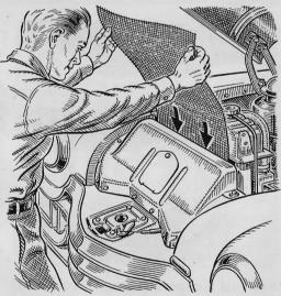
**Screen Catches Bugs.** Insects wedged within a radiator core may reduce its cooling efficiency. To keep them out, Richard C. Schneeloch, of Tulsa, Okla., suggests placing window screening between the core and grille. Clean it off occasionally.
