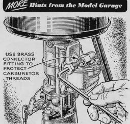
Connector Saves Carburetor. On most cars, a brass connector screws on the carburetor body, and the gas line in turn fits into the connector. If this brass fitting is missing from your car, installing one now may save you the cost of a carburetor later. A new one might be the only way out if a mechanic should strip the threads in the carburetor body while trying to connect the fuel line directly.
