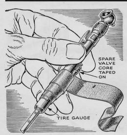
**Keep Valve Core Handy.** Place a new tire-valve core against the body of your tire gauge and wrap tape around it. The core may come in handy sometime if you find a leaking valve while checking your tire pressures.
