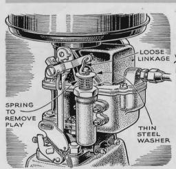
Spring Helps Pickup. In older cars there's sometimes a slight delay before the engine responds to pressure on the accelerator. This results from wear in the linkage between the accelerating-pump lever and push rod. A coil spring and washer installed on the push rod as shown will take up the slack in the linkage.
