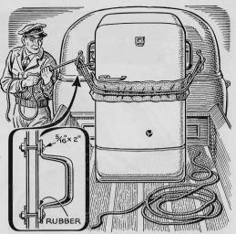
Tying Down Your Cargo. After a refrigerator had fallen from his pickup truck, Howard Butt, of Pocahontas, Va., decided it was time to stop such accidents. He bought some of the chromium handles designed to help a driver climb to his seat in a cab-over-engine truck and attached them to his truck as shown above. They made excellent tie-downs for lashing on the load.
