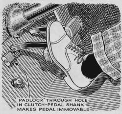
since doing it would make him conspicuous. Locking the clutch pedal is an effective way of protecting a standard-transmission car. Without the clutch the car can't be driven, and there's no easy way to saw off the lock if you drill the hole near the floor.
