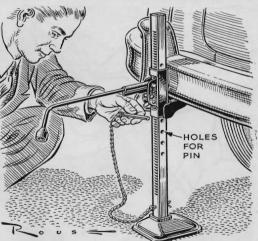
Pin Makes Jack Safer. Drill several small holes through the shaft of your bumper jack. Then, after the car has been raised to the desired height, put a steel pin through the hole under the ratchet mechanism. If the mechanism slips, the pin will keep the car from falling. The pin can be chained to the jack.
