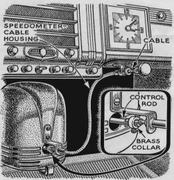
Dash Knob Controls Heater. A salvaged piece of old speedometer cable can be used as a dash control for a gasoline heater. Remove the control knob and fasten it to one end of the cable. Attach the cable to the control rod with a setscrew collar. Pushing or pulling to different positions controls the heater.
