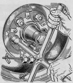
**Store Nuts on the Wreneh.** Drill a hole through the center of your four-way wheel wrench and put a toggle bolt in it. As the wheel nuts are removed, they can then be stored on the toggle bolt—safe from getting lost or filled with dirt.
