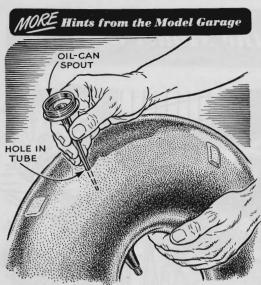
**Spout Marks the Hole.** John H. Miles, of Springfield, Mo., suggests this trick. When the tube has been pumped up and the leak located, push the oil-can spout through the hole. The tube will deflate and the spout will mark the hole.
