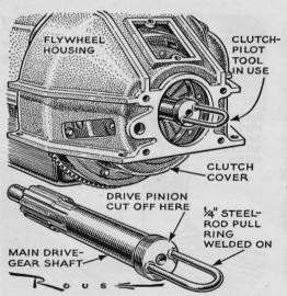
**Tool Lines Up Clutch Disk.** To assemble and disassemble a clutch, it's a common practice in many garages to use a main drive shaft from an identical transmission as a line-up tool. M. F. Sproule, of San Antonio, Tex., suggests that this will be easier to handle if you cut off the pinion and weld on a pull ring as shown.
