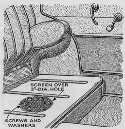
Air Outlet Improves Heater. In some of the newer cars, fresh air is delivered to the passenger compartment while the heater is running. If the windows are closed, air circulation tends to slow up. W. M. Dierks, of Chicago, found that he got improved circulation after placing a screened outlet vent under the rear seat.
