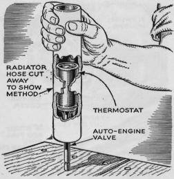
Valve Taps 'Stat in Place. An engine valve makes a handy tool for inserting or removing an inside-hose type of thermostat. Pick a valve that will just fit inside the hose. Push it in until the head rests against the 'stat. Then, with the hose in an upright position, tap the valve stem on your workbench or floor.
