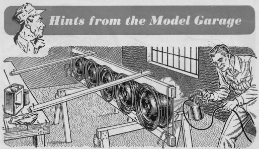
Remove Wheels for Spraying. Instead of masking the tires while you are spray-painting a car, Victor Jensen, of Bellingham, Wash., suggests removing the wheels and demounting the tires. Then set up and clamp the rims between a couple of
