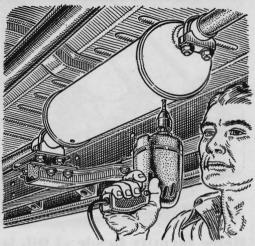
Drain Holes Save Muffler. your new muffler doesn't have drain holes, drill a couple of small ones in the places shown in the sketch. These will allow water and condensation to drain out, reducing the likelihood of the muffler rusting.
