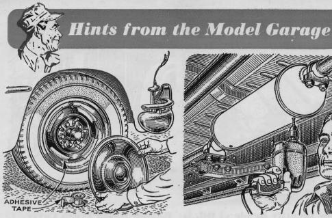
Stones in Your Hub Caps? On gravel roads, small stones can fly through the slots in the backs of the wheels and rattle around in the hub caps. To keep them out, Alvin G. Gunter, of Rockford, Ill., suggests putting tape over the slots.
