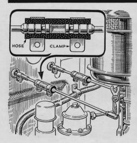
**Repairing Ford Controls.** In recent years, Fords have had molded rubber links on the hand-throttle and choke-control rods near the carburetor. Age, oil, and heat sometimes cause these to break. As a replacement, E. J. Novak, of Omaha, Nebr., suggests clamping a piece of hose on the rods. Air hose of ¼" inside diameter is just right.
