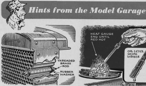
Stopping a Radiator Leak. When a leak developed in one cell of his honeycomb type of radiator, Joseph C. Cappetta, New Haven, Conn., stopped it as shown. The brass pin must be longer than the depth of the cell. The rubber washers seal the leak.
