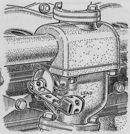
Homemade Balance Weight. When the balance weight on his manifold heater broke off, Sidney E. Lang, of Bakersfield, Calif., made his own as shown. After bolting a piece of plumber's strap around the control rod, he formed a loop in the other end, adding just enough lead to keep the valve open while the motor was cold.
