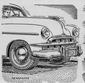
Paper Tests Brakes. Not sure which of his front brakes was grabbing, Lewis A. Emswiler, of Etna, Ohio, placed several sheets of newspaper on the garage floor in line with the wheels. Driving on the paper, he applied the brakes. The wheel with the grabbing brake ruffled the paper. It remained smooth under the other,
