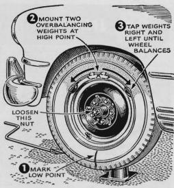
**Balaneing a Wheel.** Paul L. Bratain, of Azusa, Calif., suggests you mount the wheel in front, loosen the bearing nut, and spin it to find the low (heavy) point. Then proceed as shown. At the high point, the weights must overbalance the low side.
