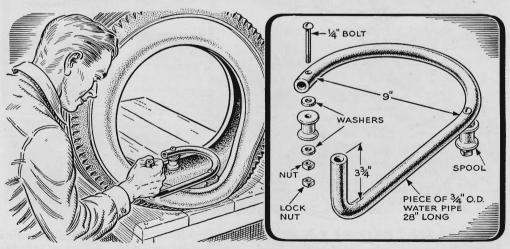
**Tire Spreader from Scrap.** If you run a repair shop, the convenience of this tire spreader will soon pay for the trouble of making it. Cut a piece of water pipe to 28" length. Bend one end to a 9" arc. The excess serves as a handle. Mount
