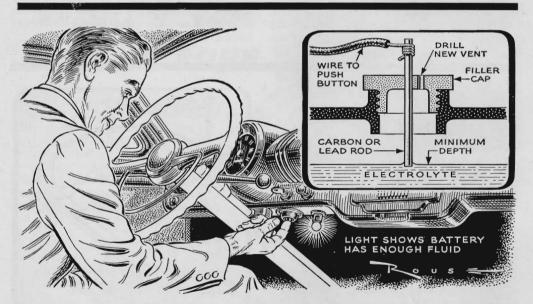
**Light Cheeks Battery Level.** To keep tabs on his battery electrolyte level during long, hot drives, Lawrence Avery, of Washington, D. C., installed a system like this. When you press the button, the bulb lights only if the fluid is still up.
