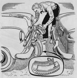
Ready for a Good Deed. Driving a new car, you may tend to pass by motorists in need of a push because your shiny bumpers might get marred. John Calder, of Laurel, Md., prepared for this by cutting two 12" lengths from a tire, trimming out the bead, and threading in a loop of wire. By hanging these on the bumper guards he can give (or receive) a push without damage to either vehicle.
