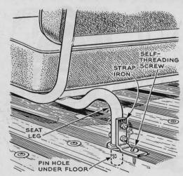
Removing Station-Wagon Seat. To remove the middle seat from recent Ford station wagons, you must crawl under the vehicle and pull out a couple of pins. To make the job easier, Marion L. Rhodes, of Knightstown, Ind., bolted a strap-iron bracket to each seat leg as shown. Removing the screws frees the seat.
