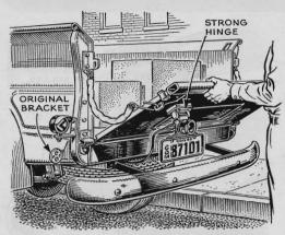
License Hinges on Tail Gate. On a pickup bought by the Modern Air Conditioning & Refrigeration Service, of Long Island City, N. Y., it was discovered that lowering the tail gate partially obstructed the tail light and license plate. A company mechanic solved the problem by mounting a hinge on the tail gate and bolting the light and license bracket to the hinge. This keeps light and license in full view.
