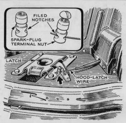
**Repairing Hood Release.** If the fitting gets lost from the end of a hood-release cable, James McElroy, of Kent, Ohio, suggests this fix. File notches in opposite sides of a spark-plug nut, pass the wire through, and clamp it with a small screw. The same idea might be used for choke and throttle controls.
