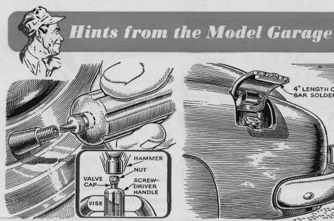
Keeping Valve Cap. A valve cap embedded in a wooden screwdriver handle keeps it handy in your tire-repair kit. Holding the screwdriver in a vise, slip a protective nut over the valve-tool end of the cap and drive it into the wood.
