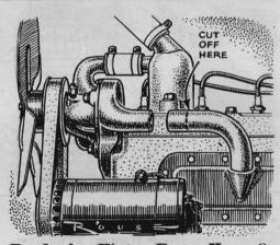
Replacing Water-Pump Hose. On a 1941 Hudson, this usually requires removal of the pump. Marion L. Rhodes, Knightstown, Ind., suggests removal can be avoided by cutting 1" off the block connection. Leave the clamps on loosely, apply sealer inside each end of the new tube, and slide it on the block connection far enough to let the other end slip on the pump outlet.
