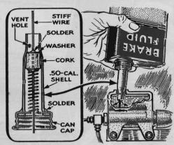
Don't Spill Fluid. A valve for filling master cylinders directly from the brake-fluid can is a useful gadget. Designed by N. E. Peeler, St. Paul, Minn., the valve keeps fluid from spilling when the can is inverted for use. It opens and the fluid is automatically released when the wire strikes the bottom of the cylinder reservoir.
