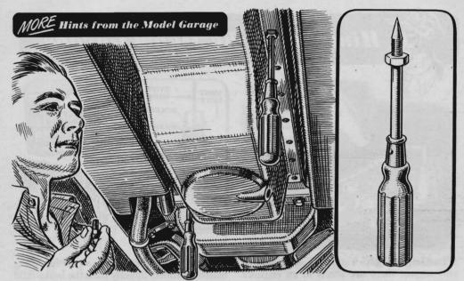
**Tired of Holding Up Pans?** Like a lot of other mechanics, John H. Miles, of Springfield, Mo., found it awkward to hold up an oil pan with one hand and start the bolts with the other.
