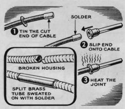
**Solder Speedometer Cable.** In some speedometer-cable replacement kits, you find instructions to cut the cable to length and attach the tip by crimping. L. M. LaBar, of West Pittston, Pa., finds it's better to tin the end (1), slip on the tip (2), and sweat it fast (3). A broken cable housing (inset) can also be repaired by tinning a split brass tube inside and sweating it on the break.
