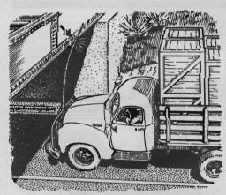
Clearance Pole Warns Trucker. If you truck tall cargo that's likely to become entangled with low bridges and wires, you might borrow an idea from the lamily cat. Attach a bamboo fishing pole to the front of the truck as a warning "whister." Make it a trifle taller than the load.
