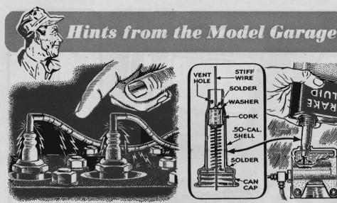
Finding High-Voltage Leaks. If you suspect there are shorts in an engine's high-voltage system, suggests John Vincenti, of Kennett Square, Pa., start it up in total darkness and take a look. You may find sparks flying from many unexpected places-wires with worn insulation, dirty plugs, or cracked distributor caps.
