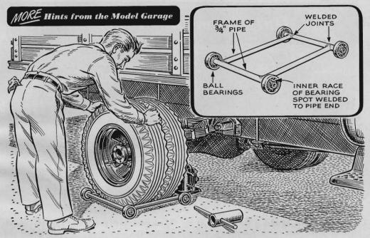
**Dolly Handles Dual Tires.** For removing and installing dual truck tires as a unit, Charles D. LaRue suggests making up a dolly like this. The original is in use at a shop in Sacramento, Calif.
