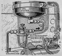
Magnet Helps Filter Oil. B. M. Thomann, of Kenmore, N. Y., finds that this setup gives his oil filter a helping hand and prolongs the life of each cartridge. It consists of a fuel filter with the element removed and a permanent magnet resting in the bowl. Considerable sediment settles out and the magnet holds fine metal particles.
