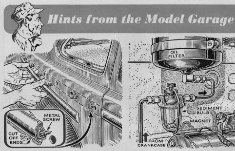
Safety Pins Hold Chrome. If a trim strip on your car has lost any spring clips, safety pins will fasten it down. Cut the ends off each pin as indicated and attach to the body metal with a self-tapping screw through the loop of the pin and into a small drilled hole. Snap the trim strip over the cut ends of the pin.
