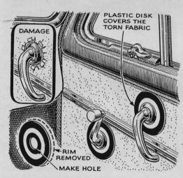
**Repairing Handle Wear.** Plastic coasters from the dime store can be used to hide torn fabric around a door handle. Cut the rim from the coaster and make a hole large enough to slip over the handle. Clamp in place with the original flange.
