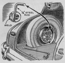
Welded Crank Loosens Spare. In some cars, it's difficult to swing the lug wrench to loosen or tighten the nut that holds the spare. J. W. Rocke, of Globe, Ariz., suggests making the job easier by welding a crank to the nut as shown.
