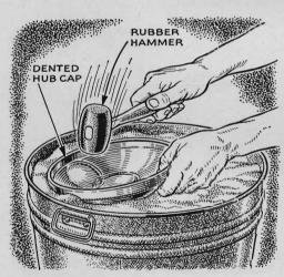
Straightening Hunb Cap. A bucket or tub of sand and a rubber mallet are all you need to bump most dents out of a hub cap. Work from the inside of the cap, using light taps and checking frequently to keep from making new outward dents.
