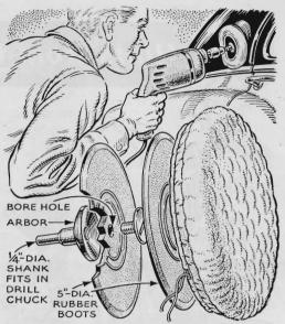
**Tire Boots Pad Buffer.** Two tire boots make excellent backing for a buffing bonnet. Use the round kind that are reinforced at the center. Run the screw through only one. The other will then prevent scratches if the bonnet wears through.
