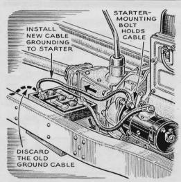
For Easier Starting. Your engine may start a lot quicker, especially in winter, if you transfer the battery ground lead from the chassis to the starting motor. With the battery grounded to the chassis, a rather high voltage drop sometimes occurs. The trick will work on both positive- and negative-grounded batteries.
