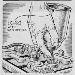
**Can Makes Valved Funnel.** Cut the bottom from one of the containers in which whipped cream is now sold and you've got a handy funnel for filling a battery. Before cutting, make sure can is empty. Pressure on the stem opens the valve.
