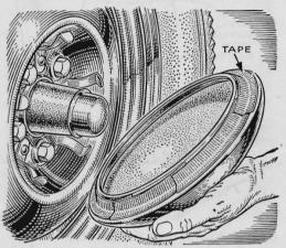
Tape Protects Wheel Paint. The outer rim of a hub cap sometimes wears paint off the wheel, leaving a rusty ring. I. C. Branstetter, of San Francisco, has found that this can be avoided by placing strips of masking tape around the rim.
