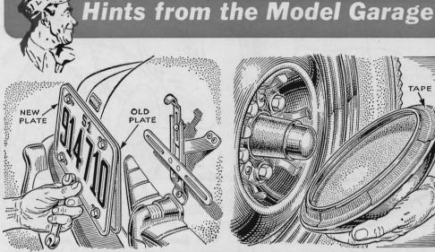
Old Plate Reinforces New One. Some states economize by making their automobile license plates out of thin-gauge metal. You can reinforce these-or any other plates -by reversing your old ones on the bracket behind your new plates.
