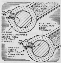
Refitting a Grease Fitting. If a grease fitting won't take grease, it may be that the end bears against the shaft, keeping the grease from getting through. Try a new fitting first. If that doesn't work, you can do one of two things-file a notch in the end of the fitting or use a washer as a spacer to hold it away from the shaft.
