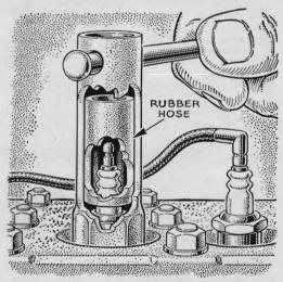
Hose Protects Spark Plug. When you are removing or replacing a spark plug, the porcelain may be cracked if the wrench slips to a cocked position while you are exerting pressure. To prevent this, Marion L. Rhodes, of Knightstown, Ind., suggests slipping a short piece of rubber inside the wrench to act as a cushion.
