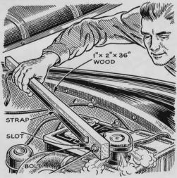
Removing Hot Radiator Caps. If a car is steaming, this job can sometimes lead to nasty burns. For his own protection, Marion L. Rhodes, of Knightstown, Ind., rigged up the tool shown above. The leather strap is looped around the cap and pulled snug. The long handle puts the mechanic a safe distance away from the steam.
