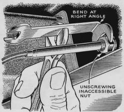
Bent Wrench Fits Tight Spot. Richard D. Briggs, of Spencerville, Ohio, reports that a wrench like this is one of his most useful tools for working in narrow quarters. To be bent this way, the wrench must be the stamped kind.
