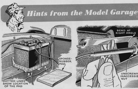
Pad Lengthens Battery Life. A rubber pad placed under a battery will protect it from jolts and jars on rough roads. Even if the hold-downs should loosen, the rubber pad will keep the battery from being damaged by the jouncing.
