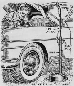
**Old Parts Make Shop Lamp.** Using scrap parts found in any garage, you can quickly make a shop lamp like this one, built in Wilmer D. Crago's shop at Red House, W. Va. The bent bolt in the pipe lets you adjust the height easily.
