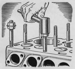
Two Nuts Tighten Stud. variation of the old two-nut trick makes it possible to use a socket wrench in reseating studs in an engine block. The washer between the two nuts keeps the wrench from slipping down over the lower one. After the stud has been seated by turning the top nut, the nuts are released by first turning down the lower one with an open-end wrench. This keeps the stud from loosening.
