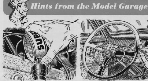
Where's the Funnel? If you can't find it, pour oil in the crankcase this way. Punch one hole in the top of the can and another in the side just under the top rim. Keep a finger over the side hole until it's in position over the inlet.
