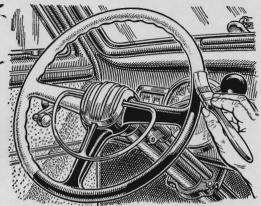
Refinishing Steering Wheel. Model-airplane dope is better than most paints for refinishing a steering wheel that tends to blacken your hands. It dries hard in a few minutes and is not affected by perspiration as paint may be.
