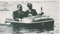
and can do up to 37 m.p.h. on land, six or seven knots in water. The vehicle weighs about 385 pounds and is made of fiberglassreinforced polyester. It was recently introduced at a Bordeaux sports show.
