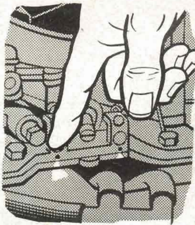
Gus pointed to a telltale patch of clean metal below a tiny passage hole drilled in the carburetor body. A loose plug in the hole allowed gasoline to trickle slowly out of the fuel bowl.
