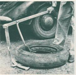
AFTER a tire has been mounted for a long time, it's often difficult to break the bead loose from a rusty rim. The homemade device shown here, which would be especially valuable in a repair shop, does the job easily. It can be quickly made from steel strap, say about 3/16" by 1½". The foot need not be as fancy as that shown in the photo. A spadelike end on the pivoted arm breaks the bead when you press the handle down. A coat of paint will keep the device from rusting.—C.A. Cole, Graham, Ala.
