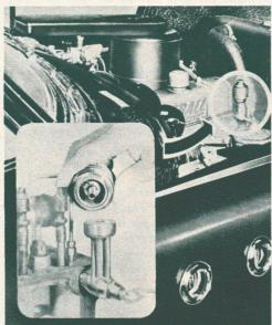
Installed in the oil line coming from the crankcase, this filter is said to help prevent distribution of damaging sludge or scale to overhead-valve parts. Termed a rockerarm oil-line filter, it's made by Ralph F. Roussey and Associates, Inc., of Chicago, and sells for about \$7.50. The filter is easily removed for cleaning.
