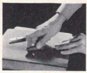
• Aloxite Brand Aluminum Oxide Cloth is excellent for producing a polished surface on metal objects and for removing small amounts of metal in fitting parts. Small flat work, for instance, is rubbed over the cloth, laid on a flat table, as illustrated. In addition to polishing metal, Aloxite Brand Cloth can be used for the removal of rust or for cleaning prior to soldering.
