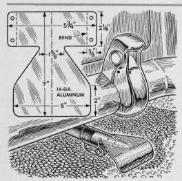
Made from one piece of 14-gauge sheet aluminum, this exhaust deflector will remain bright and rust-free while it directs hot exhaust fumes down toward the ground. Clamp it to the tailpipe with two bolts and bend the outer end down slightly.
