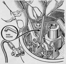
A piece of wire solder will guide a small nut onto a bolt where your finger can't reach. Thread the nut part way on the soft solder and place it against the bolt end, where a wrench can turn it off the solder and onto the bolt.
