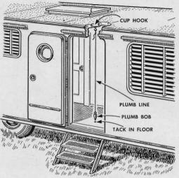
Set up a trailer once with a carpenter's level to install this leveler. Then suspend a plumb line from a cup hook screwed into the ceiling and drive a tack into the floor beneath the point of the plumb. All future leveling can be done by hanging the line on the hook and shifting the trailer until the plumb bob hovers over the tack.
