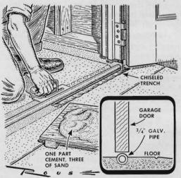
To keep rain, leaves and dirt from blowing under your garage door, install a length of galvanized pipe across the threshold. Chisel out a trench from jamb to jamb about half the diameter of the pipe, lay the pipe in place and trowel concrete flush with the floor on both sides.
