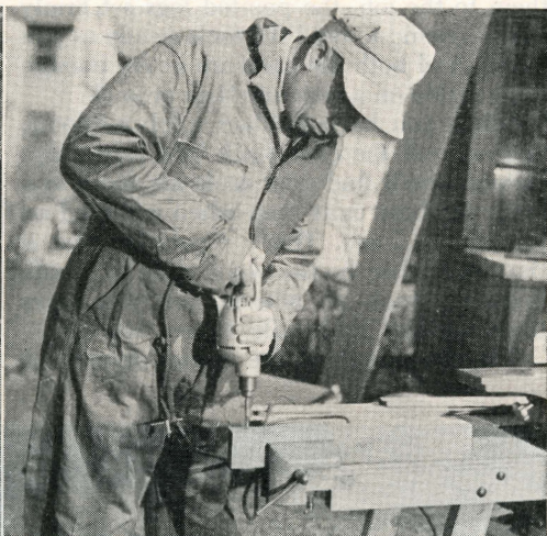
Vise on corner of jointercart worktable is handy accessory. Since jointer isn't flush with side of frame, vise can handle long work.
