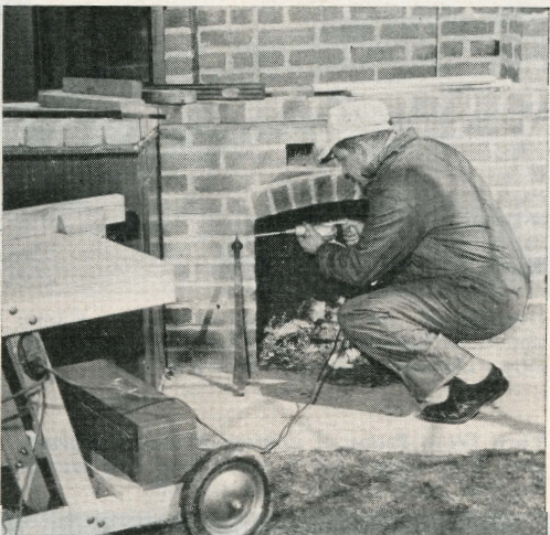
Triple outlet on leg of jointercart saves trouble of disconnecting and connecting main extension cord when drill is used.
