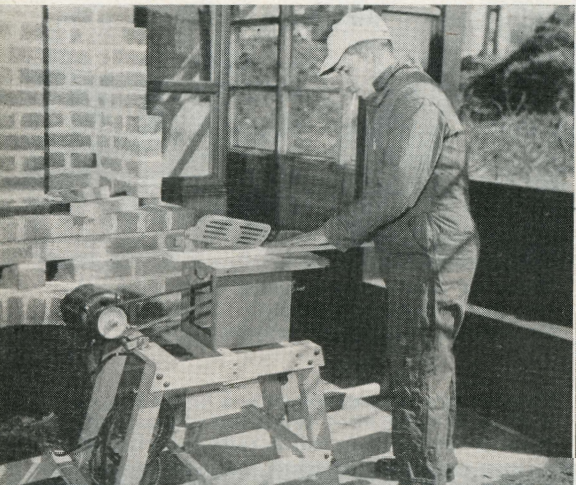
Saw in use. Even on hard surface like concrete walk, both units are heavy enough, and have legs spaced sufficiently, to be completely stable.
