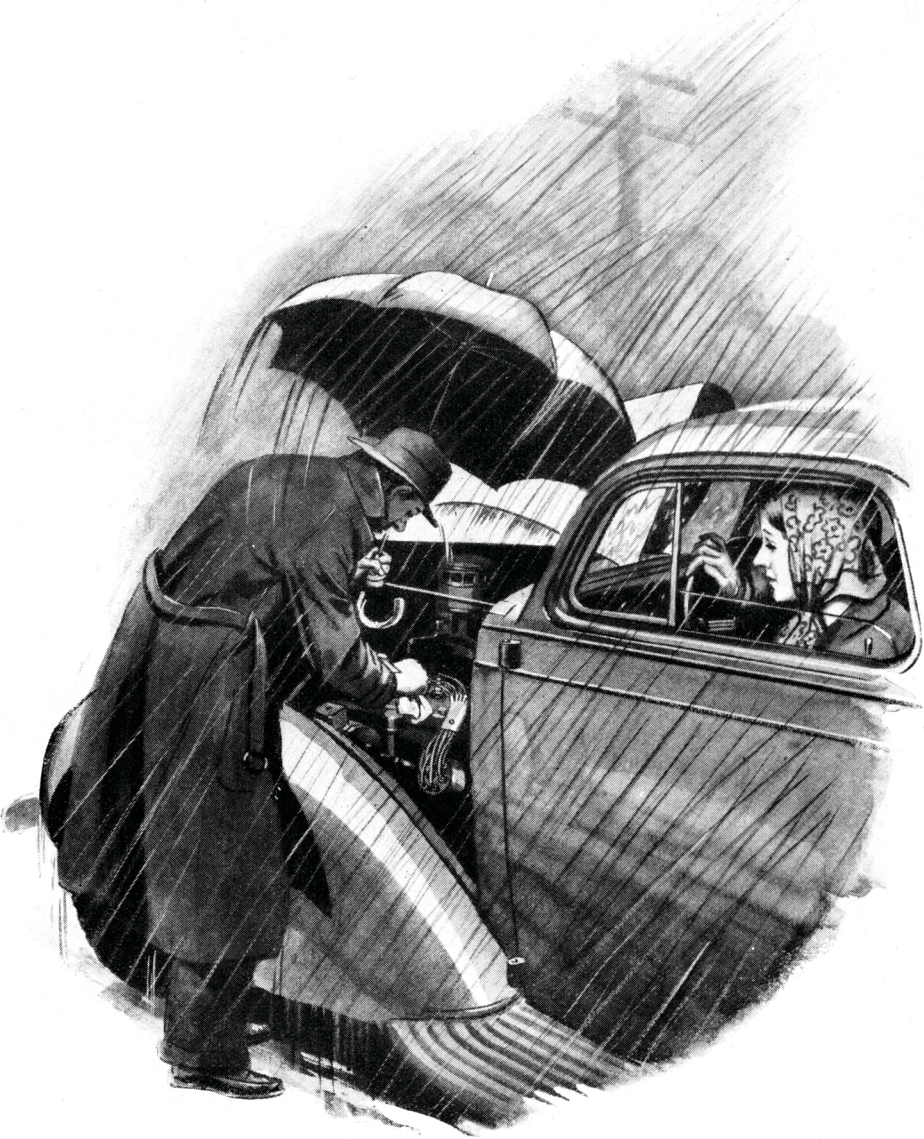
Holding the umbrella so that it protected the motor as well as himself, Devon carefully wiped off the insulator of each spark plug and then the surface of the electric cable leading to it
