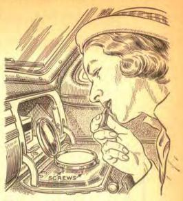
Mirror Is Always Handy. Here's the way W. M. Dierks, of Chicago, filled the bill when his wife asked for a convenient mirror for use in the car. Buying a large compact, he mounted it as shown inside the glove-compartment door, drilling holes and attaching it with screws. While not in use, the compact is kept closed.
