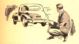
Do the wheels track? Rear wheels should follow front ones squarely. You can tell by riding behind the car or watching as it is driven off. Also note whether the wheels wobble, which can be a sign of a bent axle.
