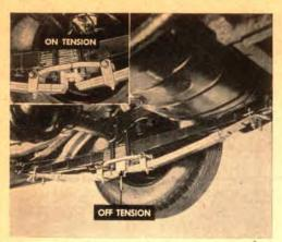
These overload springs don't cause hard riding after trailer is unhitched. Swiveling the H-shaped block removes or applies tension. The makers also offer releasable leaf-spring helpers for cars with coil springs. Another manufacturer sells helpers that adjust to suit the load.
