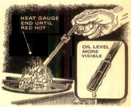
Oil Line Shows Better. To make the oil line more visible on your crankcase dipstick, Edward Wujcik, of Detroit, suggests heating the gauge end red hot in a gas flame and then letting it cool. The heat changes the color of the stick.
