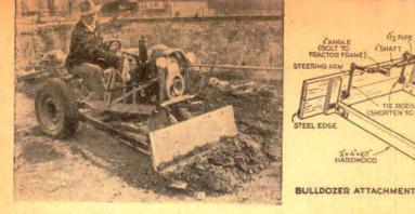
Homemade bulldozer attachment hangs on rear axle of tractor. As the sketch shows, Matous
