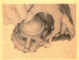
Flex diaphragm to its full stroke when tightening the flange screws. For square seating, alternately tighten screws directly opposite.
