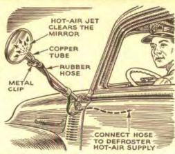
Defroster Clears Mirror. sleety weather, Ronald Weller, of Jerseyville, Ill., found that the rear-view mirror on his truck frequently became coated with ice. To keep the mirror clear, he ran a rubber hose from the defroster out to the mirror.
