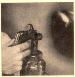
Lay a smooth surface for the finish coat by applying the primer with a spray gun. Follow the priming coat with wet sanding. You'll get a better job by refinishing the entire fender.
