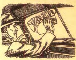
Eraser Cleans Windshield. George A. Smith, of Quarryville, Pa., suggests that a clean blackboard eraser is a handy item to carry in your glove compartment. When moisture collects on the inside of the windshield, a few strokes with the eraser will quickly give you unobstructed vision.
