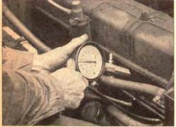
1. A compression test comes first. An engine cannot be tuned satisfactorily if compression is uneven. In such cases, a valve or a ring job may be required before the tune-up.
