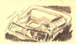
Noise in the differential? To check the rearaxle assembly, ride in the rear seat or, better still, remove the rear-seat cushion. On a smooth road (preferably a smooth blacktop to lessen tire noise), pick up speed slowly and evenly to about 50 m.p.h. with your ear cocked to the rear. Then shift into neutral and coast to a stop. Should you hear any grinding, knocking, or hum from the rear end, a heavy repair bill may be in the offing.
