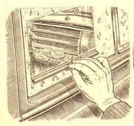
Clearing Fogged Windows. Richard H. Hanson, of Melrose, Mass., makes it a practice to carry an extra windshieldwiper blade. Besides serving as a spare in case of loss of one of the regular blades, it also comes in handy as a squeegee for clearing fogged windows. It's also useful for drying the windows after a car wash.
