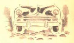
Do the wheels shimmy? Drive over a rough pavement, the rougher the better. If the wheels shimmy, it may come from at least a half-dozen causes. Repairs are liable to be troublesome and can be costly.
