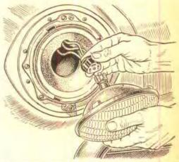
Corrosion Knocks Out Lights. If either beam of a sealed-reflector headlight goes out, be sure you really need a new unit before putting down the cash. In some cases, particularly in older cars, you will find the contacts have become so corroded that the resistance prevents the lamp from lighting. Careful cleaning of the contacts will restore the light to usefulness.
