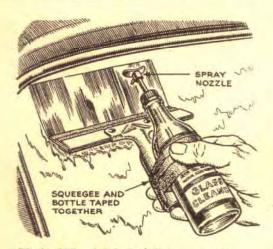
Unit Windshield Cleaner. Tape a rubber squeegee to a bottle of glass-cleaning fluid fitted with a spray nozzle, writes Sally Mills, of Syracuse, N. Y. When the windshield needs cleaning you only have to dig out the one unit to spray the fluid and wipe it off immediately.
