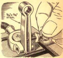
Wedge Loosens Battery Clamp. T. E. Waters, of Atlantic, Iowa, made this wedge to open up stuck battery clamps. The chisel-shaped end is tapped between the clamp's ears. Then the thumbscrew is turned to spread the clamp apart.
