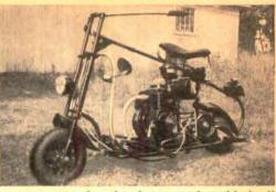
water pipe for the frame and welded all joints. Fittings are made from flat and angle iron. Clutch action is obtained through a jackshaft located just behind the motor. The shaft, which swivels in a horizontal plane, is moved by a pedal to slacken or tighten the drive belts in operation.
