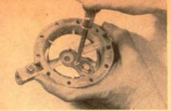
Install new valves and gaskets exactly as old ones came out. Watch whether large or small end of each valve cage goes down or up.
