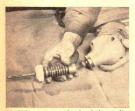
11. Valve seats are refaced with this grinding tool, shown in use on page 180. The protruding stem keeps the stone and seat in proper relationship. The grinder has a 45-deg. face.
