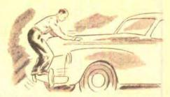
Test the shocks. Jounce on the front and rear bumpers. If the car continues to bounce after you jump off, the shocks need repair, or perhaps replacement. (This also tests the bumpers themselves for tightness.)
