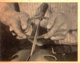
TEST THE RING in the bore, pushing it down with the piston to be sure it isn't cocked, Insufficient and gap will cause heat to buckle it
