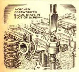
Tappet Adjustment Is Easier. It is usually recommended that the tappets of an overhead-valve engine be adjusted while the engine is warm and idling. However, you've probably found that it's hard to keep the screwdriver in position on the bouncing adjusting screw. To simplify the task, W. M. Dierks, of Chicago, filed a wide notch in a screwdriver blade. This keeps the blade in the slot while adjustments are made.
