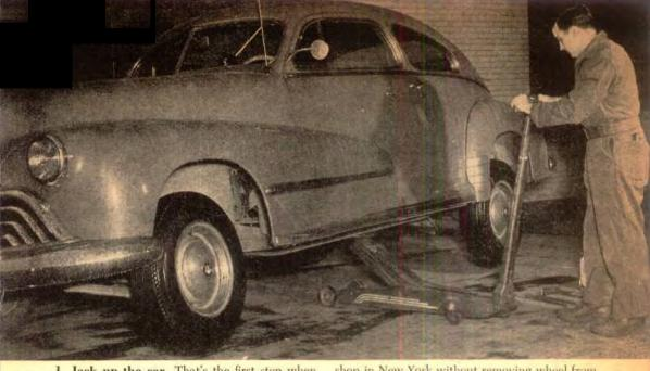
1. Jack up the car. That's the first step when tires or tubes are fixed at the General Tire
