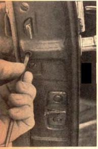
Door handles of this type are removed by loosening one setscrew in the edge of the door. Once out, the handle can be disassembled and the lock barrel removed if it should require adjustment, repair, or replacement.
