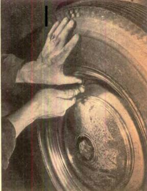
9. Some air, and job's done. Holding the stem with his thumb, he puts air in the tire before removing jack. This job took less than 4 min. Some mechanics in the shop work still faster.
