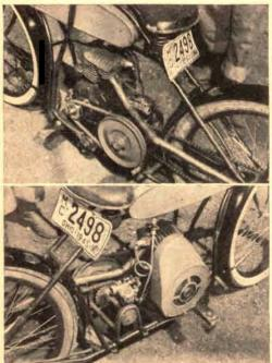
Motorbike Built from Scrap. Cast-off parts that he found lying around his father's machine shop became the raw materials for Robert Barr's lightweight motorcycle. A washing-machine motor, to which he added a carburetor for smoother performance, gives Barr a top speed of better than 40 m.p.h. Wheels, front assembly, and coaster brake were salvaged from old bicycles, and additions to the frame were made of \$" gas pipe. Drive pulleys and chain sprockets give a ratio of 6 to 1.
