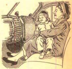
Rubber Pad Protects Kids. Sudden stops often result in bumped heads. A foam-rubber seat pad and two suction cups, mounted as shown, makes a practical dashboard guard. At the upper corners of the pad, punch holes with an ice pick. Tie heavy cord to each cup and run the cord through the holes. Large knots will hold the pad in place.
