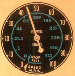
A safety feature would be the inclusion of stopping distances on the speedometer dial, reminding the driver how they shoot up as speed increases. The distances shown are for optimum conditions—halting the car on dry concrete. Slippery pavement or faulty brake action could skyrocket the figures.
