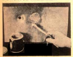
New powdered-aluminum products with a doughlike consistency are now being marketed as a substitute for solder in repairing damaged auto bodies and fenders.
