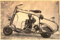
Scooter Takes Hills Easily. Employing a reduction of about four to one from motor to driven wheel makes this little scooter an excellent climber. Since it uses a 2.3-hp. engine, it still has enough power to cruise at 35 m.p.h. The Rev. J. Karlton Dewey, who built the machine, used ½"
