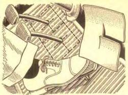
Floor Pads Stop Drafts. Wind that blows in around the shafts of the clutch and brake pedals can be stopped by pieces cut from an old inner tube or step pad, F. W. Marasco, of McKeesport, Pa., writes that it isn't necessary to secure the slit pieces if you cut them large enough.
