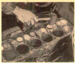
8. Using a mallet, he taps the valve head after it has been raised by the lifter. This loosens the keys for removal. Unless it is stuck, the valve can now be lifted out with the fingers.
