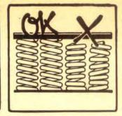
Use one new spring, if possible, when checking length and tension with the aid of a straightedge
