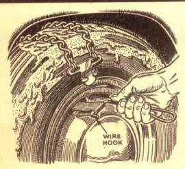
Hook Aids in Attaching Chains. Putting on strap-on chains—sometimes called mud hooks—usually is a messy and difficult job. To save my fingers and time, I use a stiff piece of wire bent to an L-shape. Most wheels have a rather small opening through which the webbed strap must pass. Run the hook through the opening and use it to pull the strap through.—John Wright, Middleboro, Mass.
