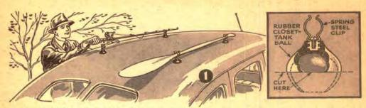
1 RUBBER VACUUM CUPS with strength enough to hold light articles on top of your car can be made from discarded flush balls that your plumber may be glad to save for you. There should be no puncture in the upper part. Cut off the balls about ½" below the halfway mark and face the edge on a rough emery wheel. Affix a spring clip to each threaded top.
