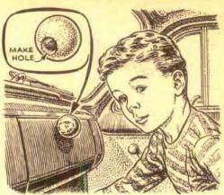
Ball Protects Children, Knobs or handles on the dash can give youngsters a bad bump on sudden stops. Sponge-rubber balls fitted over the protruding parts reduce this hazard. A dab of gasket shellac in the hole will attach the ball securely.
