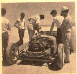
Radiator is eliminated to sharpen nose of this model. Instead, it has a 10-gallon water tank behind engine. Car is drained after each run and takes an hour and a half to cool off.
