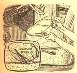
Curved Needle Mends Rips. Henry Zave, of Chicago, offers this hint for keeping your car's seat covers and upholstery in repair. Use a curved upholsterer's needle for easier sewing. You'll find this type of needle lots simpler to handle. It's especially good when you have to work from only one side of the material.
