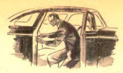
New paint may hide a former bright taxi color, Pry up the windshield seal or scratch down to bare metal on an inconspicuous part of the body to see if there's paint of another color. Has lettering on the doors been painted over?
