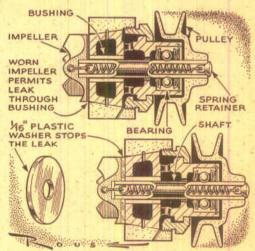
Washer Tightens Worn Pump. In overhauling a Ford "60" water pump, John Salzillo, of Brooklyn, N. Y., found that the edge of the plastic impeller had worn so much that the spring couldn't pull it snug against the pump housing. To take up the slack, he removed the impeller, and slipped a plastic washer on the shaft. This had the effect of building up the worn impeller. He cut the washer from 1/16" plastic.
