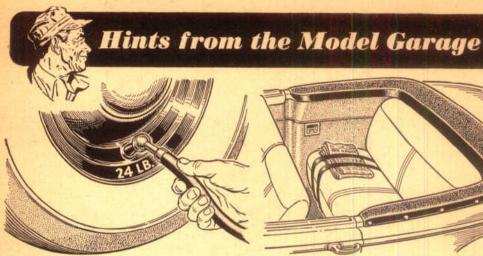
Prevent Overinflation. The new low-pressure tires are sometimes overinflated through carelessness. As a reminder to service-station attendants, paint the correct pressure on the rim beside each valve stem with white enamel, or apply waterproof adhesive tape with the figure inked on. You can also buy markers for your caps.
