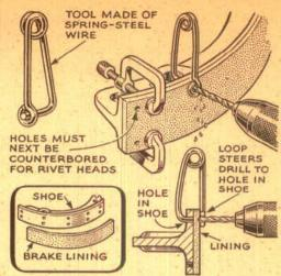
Aligning Holes in Lining. If you cut and fit lining to brake shoes, this tool will help you align the rivet holes in the lining. After the lining has been cut, attach it securely to the shoe. Then place the prong of the tool in the shoe rivet hole and drill through the tool eye. Counterbore for the rivet heads.
