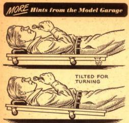
Turn Creeper by Tilting. On rough garage floors, it's often difficult to turn the usual shop creeper when you want to move to a new position. The creeper will work better if you set one pair of wheels back 12" or so from the end. Then, by shifting your weight, you can tilt the creeper slightly when you want to turn.
