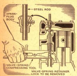
Replacing Valve Springs. This tool makes it easier to replace an intake-valve spring on an L-head engine without removing the head. It's used by adjusting the steel rod until it bears on the head of the closed valve. Turn the body into the spark-plug hole without forcing it, The spring can now be compressed and the retaining key removed. Marion L. Rhodes, Knightstown, Ind., developed the tool.
