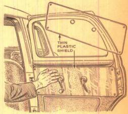
Plastic Keeps Door Clean. Most everyone these days installs seat covers in a new car, but few give any thought to the door areas, where hands frequently soil the covering material. Frank J. Montemuro, of Philadelphia, is one person who does. Cutting a sheet of clear plastic to fit, he installed it as a shield around the door and window handles on each door. The plastic is easily wiped clean.
