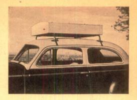
pine. Joint one edge of the stock and cut the pieces to finished length. Lay out the curve on each end and bandsaw to outline. Then clamp the pieces together and sand or plane smooth any irregularities.
