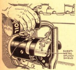
Shield Protects Generator. While filling up with oil, you may have noticed that the attendant sometimes allows a little to slop over the filler tube. Ray Wolfram, of Chicago, writes that he finally traced a mysterious generator trouble to such carelessness. Spilled over the generator, the oil had fouled the brushes. To prevent this from happening again, he installed a metal shield as shown.
