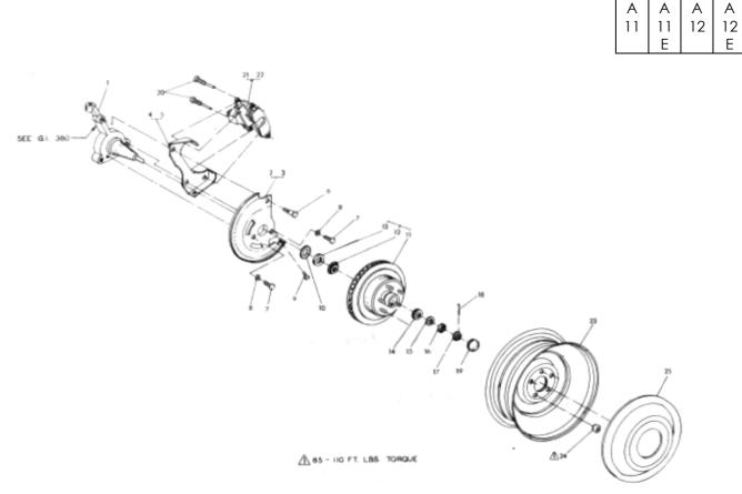
Figure 6-1 Front Hub & Rotors, Wheels, Covers Plus Associated Parts
