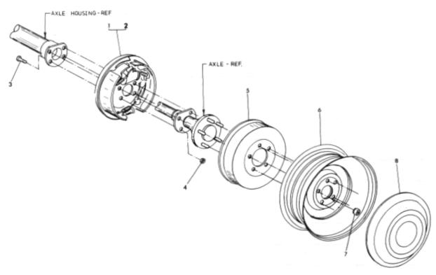
Figure 6-2 Rear Drums, Wheels, Covers Plus Associated Parts
