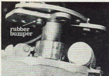
A stop pin, moving in a slot, limits the advance of the breaker plate in Delco distributors. The rubber sleeve or bumper on the pin is meant to eliminate possible rattles. But if the rubber fitting falls off, the pin permits spark advance beyond the manufacturer's specifications.
