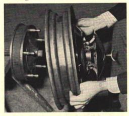
Changing auto wheels will become a simpler and speedier job if a new fastening device lives up to the claims of its inventor, Lothar Stanetzki, of Bonn, Germany. Five threadless bolts on the brake drum enter holes in the wheel, as shown above, and are grasped securely by five plierlike levers that are locked by pushing in on the hub cap. The gripping action is said to increase with the motion of the wheel.
