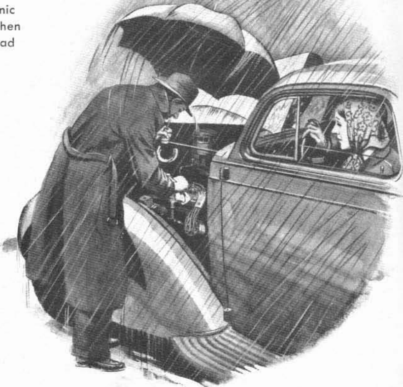
Holding the umbrella so that it protected the motor as well as himself, Devon carefully wiped off the insulator of each spark plug and then the surface of the electric cable leading to it
