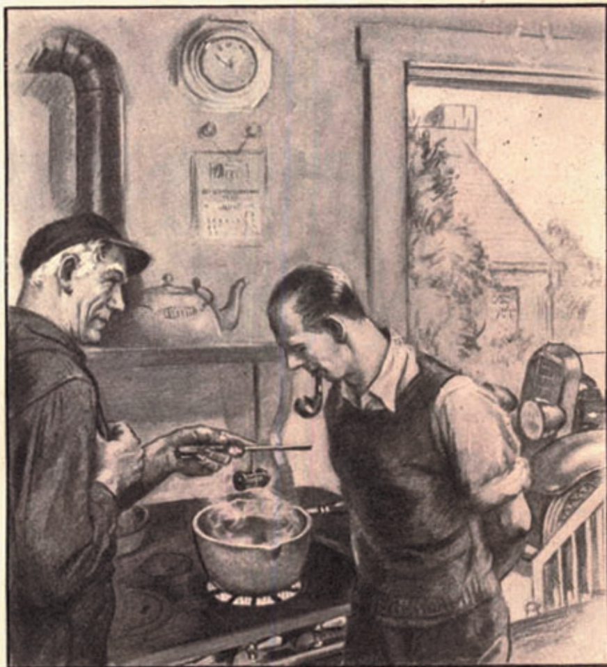
"At ordinary temperatures," said Gus, lifting the thermostat out of the hot water. "that valve is closed tight. When it's working as it should, it is wide open at 180 degrees"
