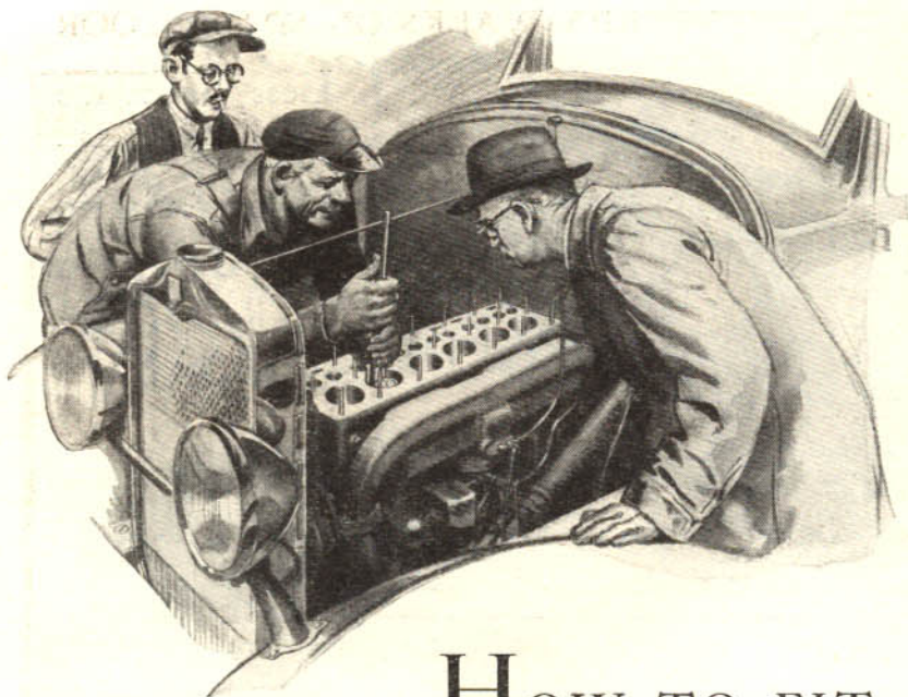
Gus, with a dial indicator gage in the cylinder, said: "See what that reads? That means the cylinders are oval, not round as when the car was new"
