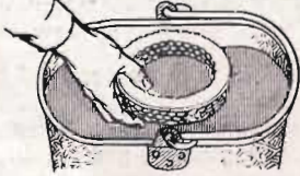
WASH ELEMENT IN CLEANING FLUID
