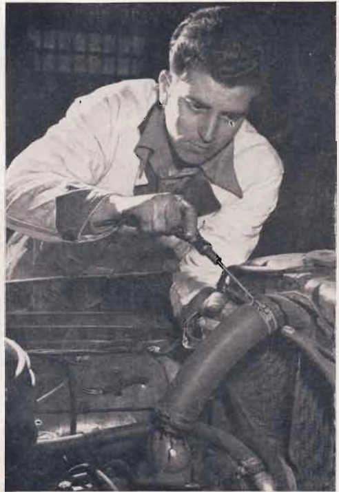
Radiator hoses are inspected and defective ones replaced. All hose clamps should be tightened carefully to prevent possible leakage of antifreeze solution
