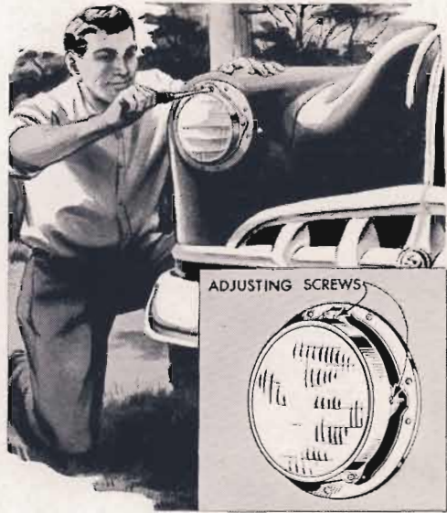
If low beam burns out, tilt both headlights downward so high beams will serve as low beams, shown above
