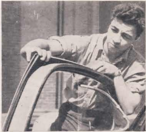
Deteriorated weather stripping on all doors can be replaced with sponge rubber to assure a tight seal
