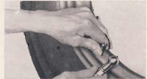
3 After the tire is fitted on the rim, inflate the tire to press the beads tightly against the rim flanges
