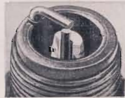
CRACKED AND BROKEN
