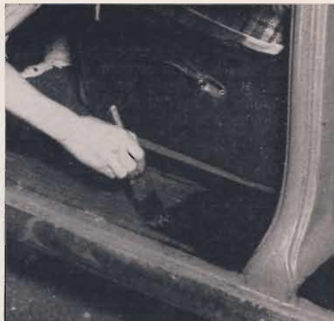
A thin mixture of drop black and turpentine makes a good dressing for the rubber mats and running boards
