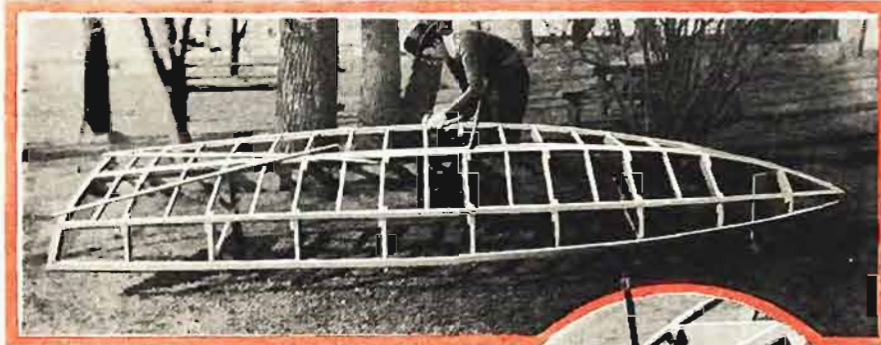
As shown in the view above, the framework is assembled bottom up on a heavy form mounted on legs like a sawhorse. The frames fit in slots in the form. At right: Planing bevel on chine.
