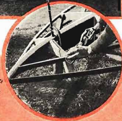
As shown in the view above, the framework is assembled bottom up on a heavy form mounted on legs like a sawhorse. The frames fit in slots in the form. At right: Planing bevel on chine.
