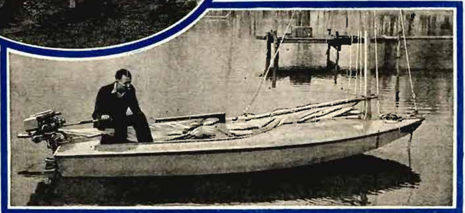
By lowering the sail and attaching the outboard motor, the combination boat is transformed into a motorboat. Insert: The side planks are applied simultaneously so as not to twist the frame.
