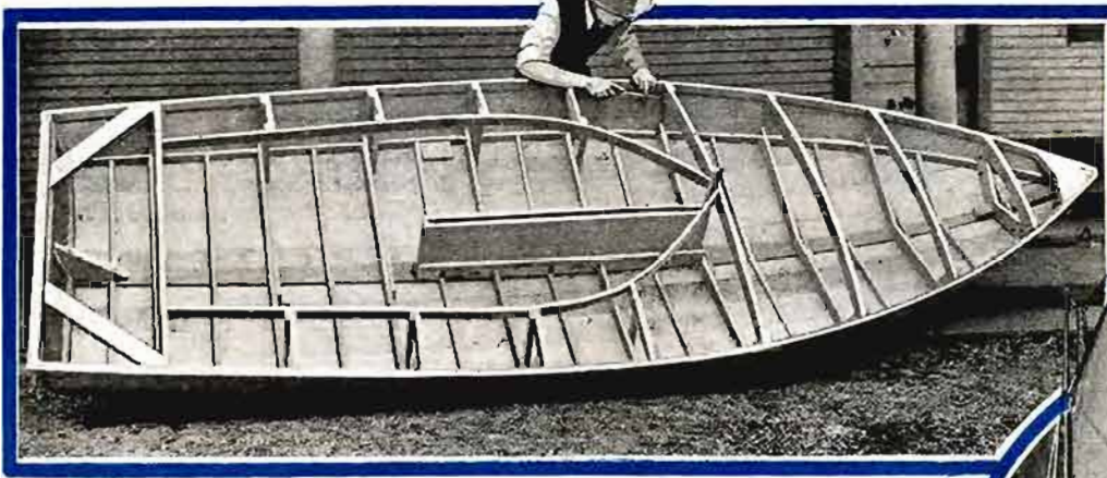
Left: An exceptional top view of the partially completed hull showing the deck frames, well for centerboard, and transom knee. Below: The author sailing his 15-ft. two-purpose boat.
