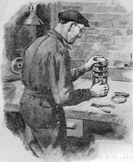
Fig. 3. A tin can with top and bottom removed aids in sliding new piston rings into piston grooves.
