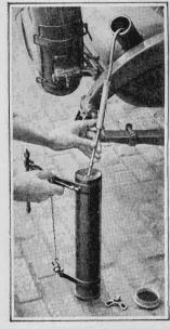
One pull on the plunger of this special gasoline tank syphon starts a steady stream flowing into the tank of the camper's gasoline stove, or into a can to help out a stranded motorist
