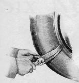
Here is a mud hook that will pull you out of a hole with It consists of a heavy. ribbed cross member with hinged side arms controlled by a bolt, so that the hook can be clamped around the tire to the edges of the rim Syphon Oil Bottle, Gripper Mud Hook, Socket Wrench Set and Other Handy Time-Savers
