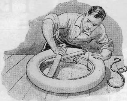
Fig. 1. An ingenious way to improve tire irons—the hooks hold the tire in place, preventing it from slipping out of your grasp
