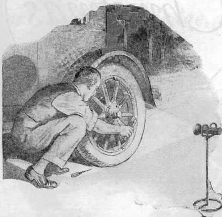
Fig. 1. A good flashlight at the correct height on a wire stand of this type will take much of the discomfort out of tire changes at night
