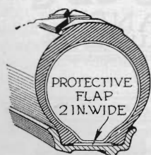
Fig. 6. A rubber band cut from an old inner tube prevents chafing
