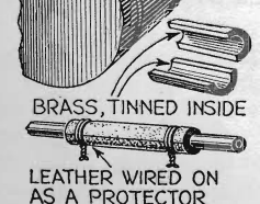
Fixing Gas Pipe
