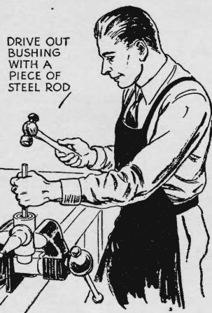
Cutting the small disk in half allows its two parts to pass one bushing so that the other can be driven out
