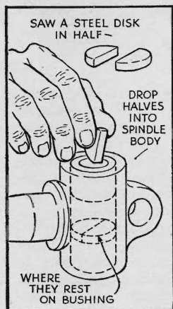
Cutting the small disk in half allows its two parts to pass one bushing so that the other can be driven out
