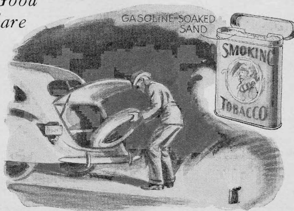
Four spools, pivoted between sheet-steel frames, make this tire spreader
